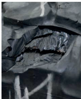
Visible damage: separation between crown plies
