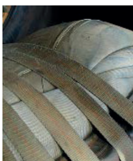
A flexible segmented press is used during cold vulcanisation tyre repairs
