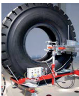
A thermopress is used during hot vulcanisation tyre repairs
