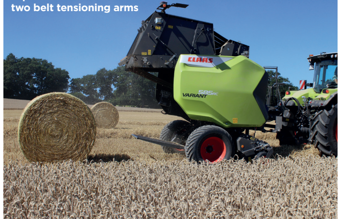
New Claas Variant 585 Roto Cut baler has separate control of the two belt tensioning arms
